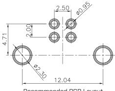
Recommended PCB Layout Top View
