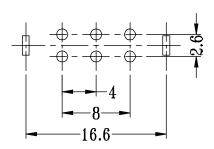
Recommended PCB Layout Top View
