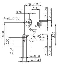
Recommended PCB Layout Top View
