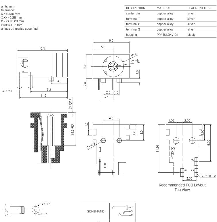
MATING PLUG Jack Insertion Depth: 8.2 mm
