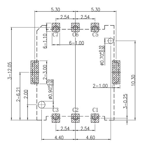
SMT SOLDER AREA Recommended PCB Layout Top View
