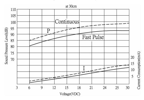
P: Voltage vs. Sound Pressure Level I: Voltage vs. Current Consumption
