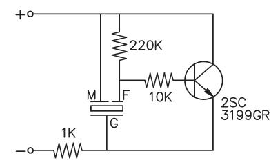
Notes: 1. The current consumption and the sound pressure level are measured by using the recommended driving circuit shown above.
