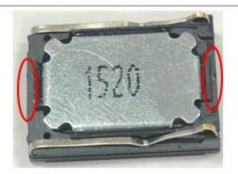
Without notches on old plastic housing. With notches on new plastic housing.
